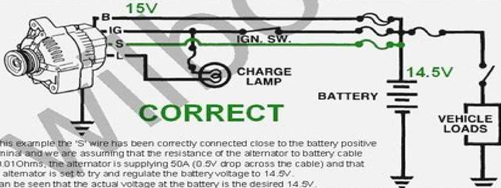
In this example the 'S' wire has been correctly connected close to the battery positive terminal and we are assuming that the resistance of the alternator to battery cable is 0.01 Ohms, the alternator is supplying 50A (0.5V drop across the cable) and that the alternator is set to try and regulate the battery voltage to 14.5V. It can be seen that the actual voltage at the battery is the desired 14.5V.
