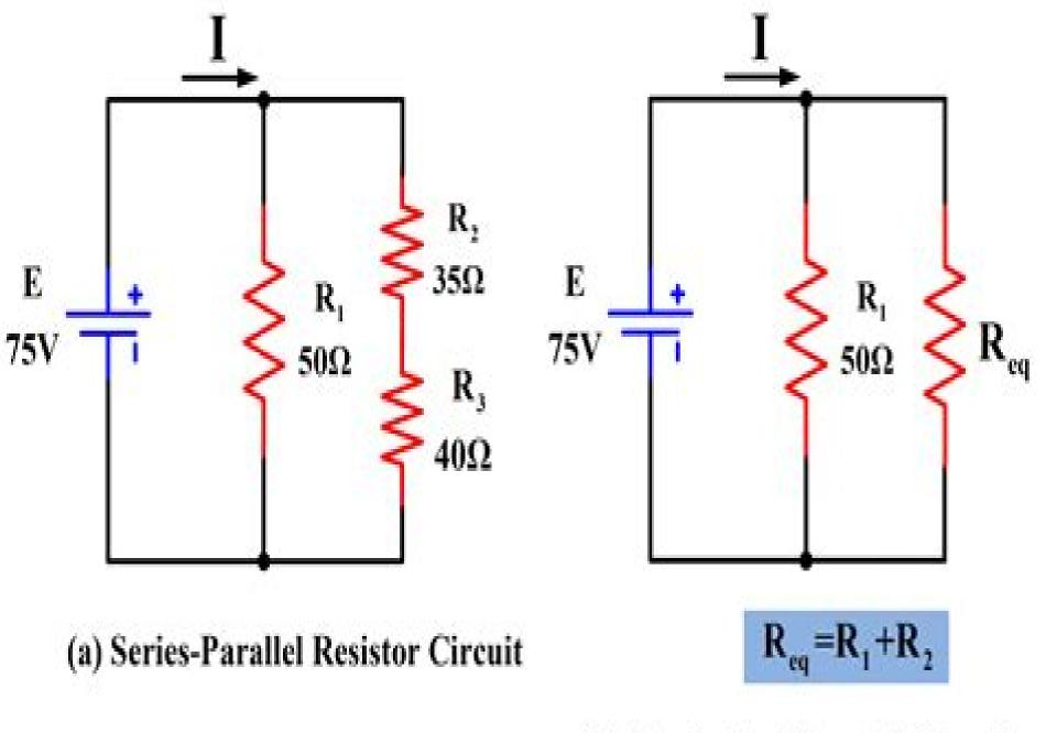
(b) Equivalent Parallel Circuit
