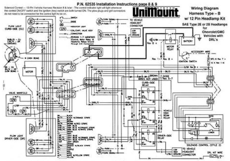
Whice harnesses – 12 pin, P.N. 61557, rev. 5, 6, or 7 – The indicator light on the solenoid control will only light when the plow is attached to the vehicle and the ignition switch and control on/off switch are both turned on.
