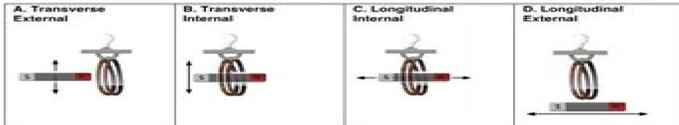
4. Move the bar magnet through the coil and observe the motion of the electrons in the forward arc of the coil loops. Report the correlations of magnet motion and electron motion.
