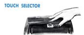
With the Touch Selector (22) on your new Sears Electric, you can adjust the tension on the typing keys to match your own typing touch. The Selector is on the bottom of the type-writer, under the Spacebar. For a light typing touch, turn the dial towards L; for a heavier touch, turn it towards H.
