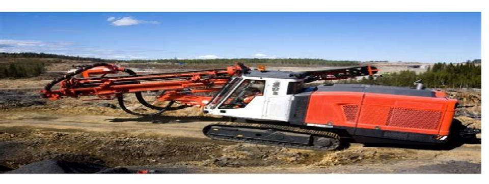
Sandvik DP1500i is intelligent, self-propelled, self-contained, crawler based surface drilling rig equipped with a cabin and a rod changer.
