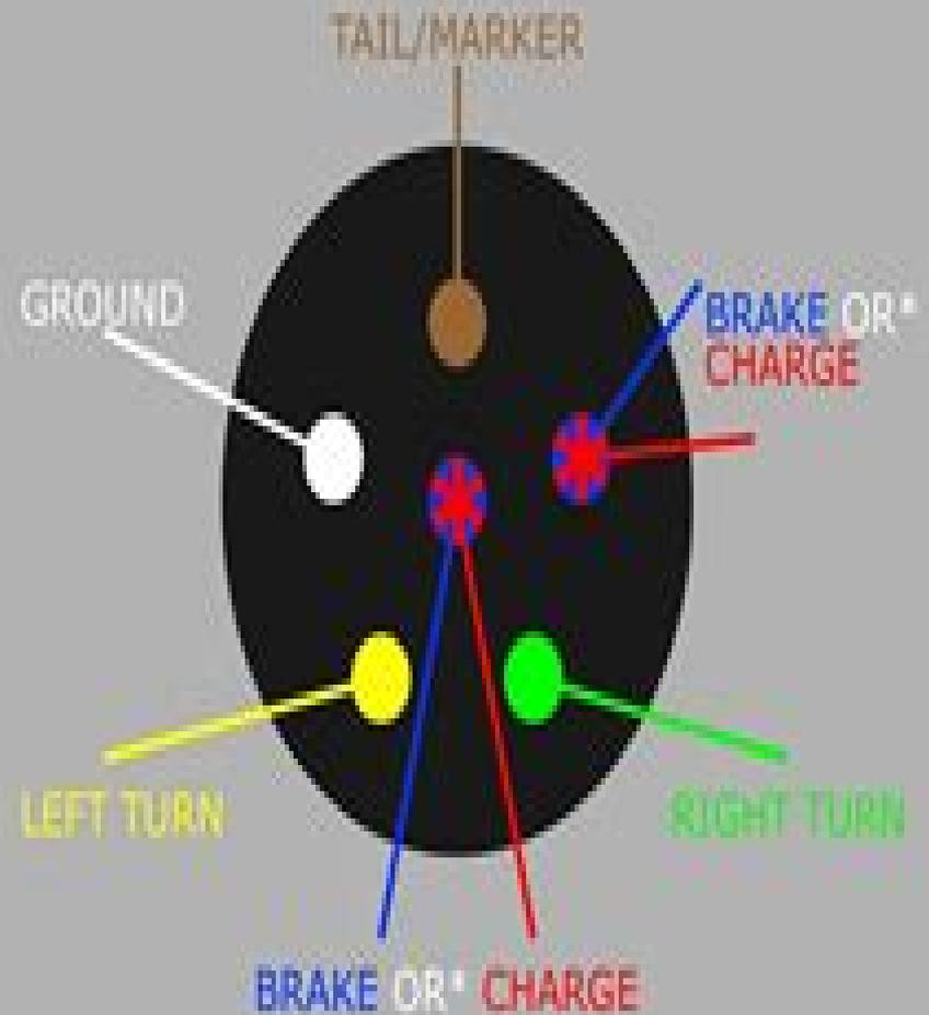
\*Brake and Auxiliary Power have two different industry standards. Identify which way your trailer is wired before wiring connectors.
