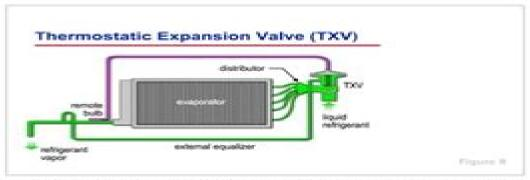
The second requirement of the refrigerant piping design is to ensure that only liquid refrigerant enters the expansion device. There are several types of expansion devices, including expansion valves (thermostatic or electronic), capillary tubes, and orifices.
