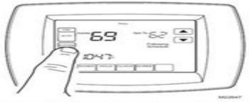
Press and hold the two blank keys on either side of the center blank key for approximately five seconds until screen changes. Release the two blank keys when the screen on the comfort control matches the screen below.
