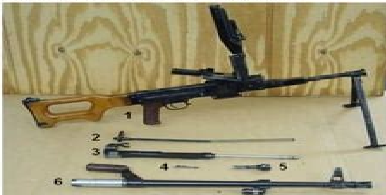
Figure 4-19. PK Machinegun Field Stripped
