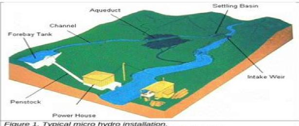
Figure 1. Typical micro hydro installation. Source: http://practicalaction.org/?id=micro\_hydro\_fag
