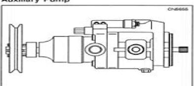
Type: Auxiliary Pump is an externally driven, splined shaft, variable piston, pressure compensated hydraulic pump.
