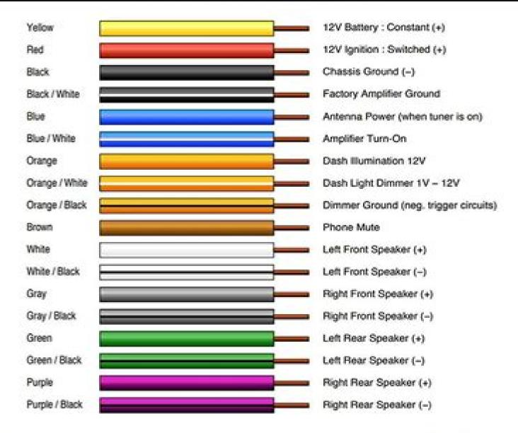
The color codes used on aftermarket car stereo connector harness's conform to the E.I.A (Electronics Industry Association) standards. These colors often differ from the wiring colors used by vehicle manufacturers. Always refer to your stereo owner's manual for specific wiring details before making any connections.
