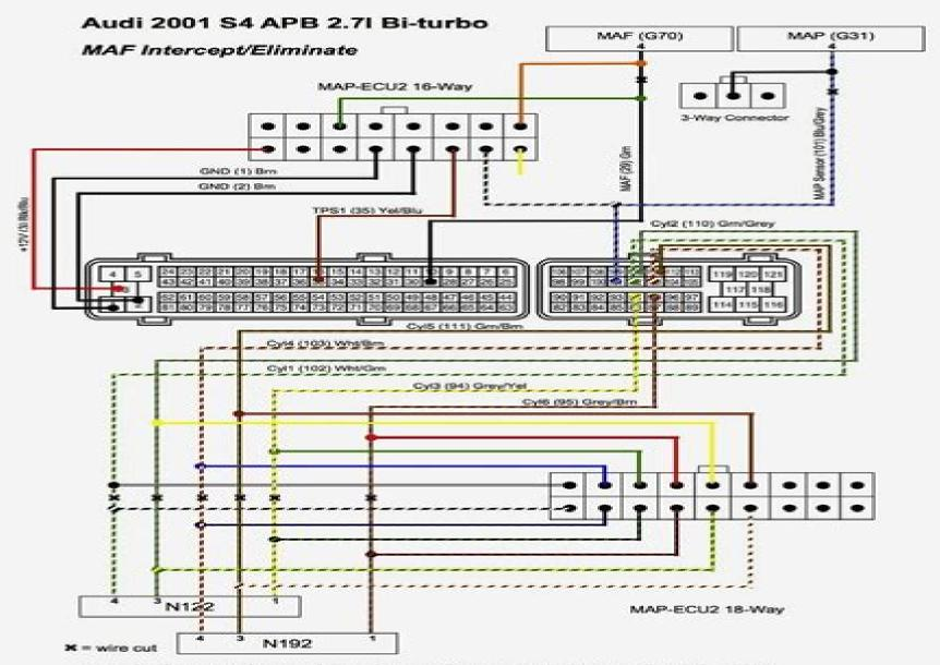
Note: Configure to 6-Cylinder Coil on Plug, MAF Intercept - MAP Y-Axis, Ext MAP = FCD1, Analog 2 Output = FCD1 for fuel out defeat (if required). Firing Order: 1-4-3-6-2-5
