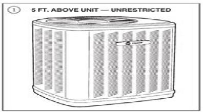
service access to meet National Electrical Code. Also, the unit location must be far enough away from any structure to prevent excess roof run-off water from pouring directly on the unit. Do not locate unit(s) close to bedroom(s).
