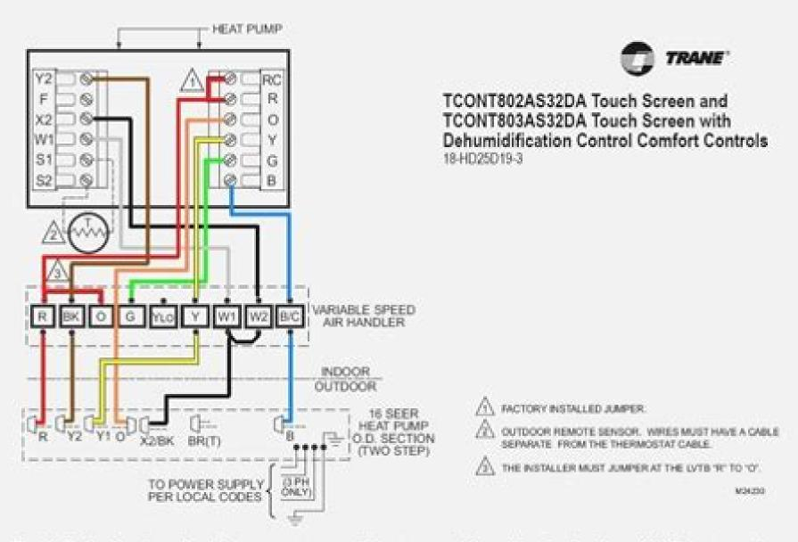
Fig. 11. Typical hookup of multistage two-step scroll heat pump with auxiliary/backup heat (3H/2C heat pump).
