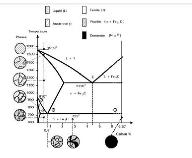
Figure 6 Iron-carbon phase diagram
