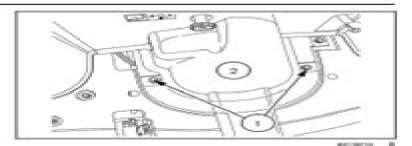
Remove the platform retaining bolts (1) from the righthand side (2) of the platform.
