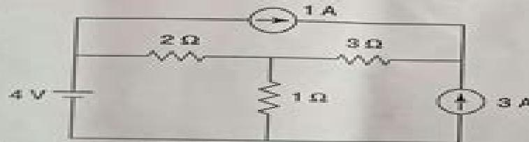
C) Define the terms : Branch and Node related to graph of a network and For the graph shown below write the (a) incidence matrix (b) Tie set matrix
