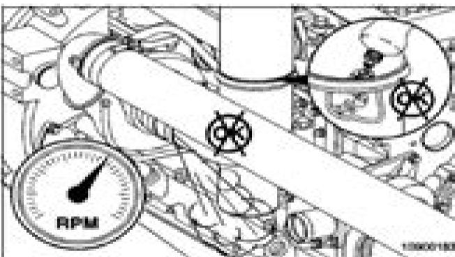
Operate the engine at full throttle and rated rpm with maximum load.
